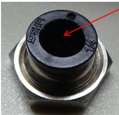
**Insert tubing** past the locking teeth and continue pushing till tubing bottoms out.
